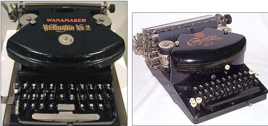
Figure 87. Wellington No.2 (1890s) and Empire No. 2 (1908) - from left to right; bars sliding forward to platen (thrust action) (Source: http://ednixon.com/pix/2003/typewriters/Pa136413.jpg and http://typewriter.rydia.net/empire2.JPG )
