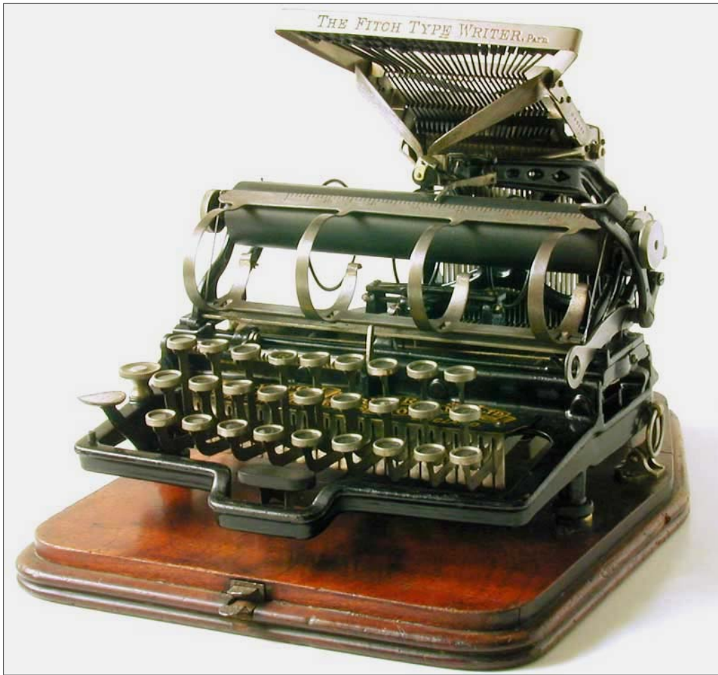
Figure 86. The Fitch Typewriter (1888); type bars standing erect and swinging down from the rear (downstrike) (Source: http://www.maquinasdeescreverantigas.com.br/fotosg/fitch-front-jpg.jpg )
