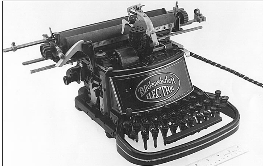
Figure 50. Blickensderfer Electric; the first electric typewriter, not marketed, c1902 (Source: http://www.precision-dynamics.com.au/typewriters/blickensderfer.html )
