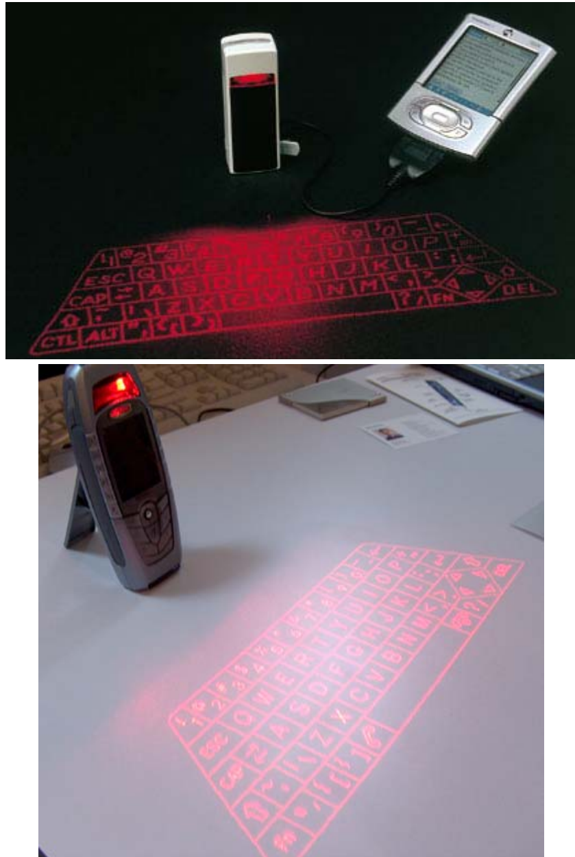
Figure 79. Examples for virtual keyboards; a Palm PC and below a Siemens mobile phone (2000s)
