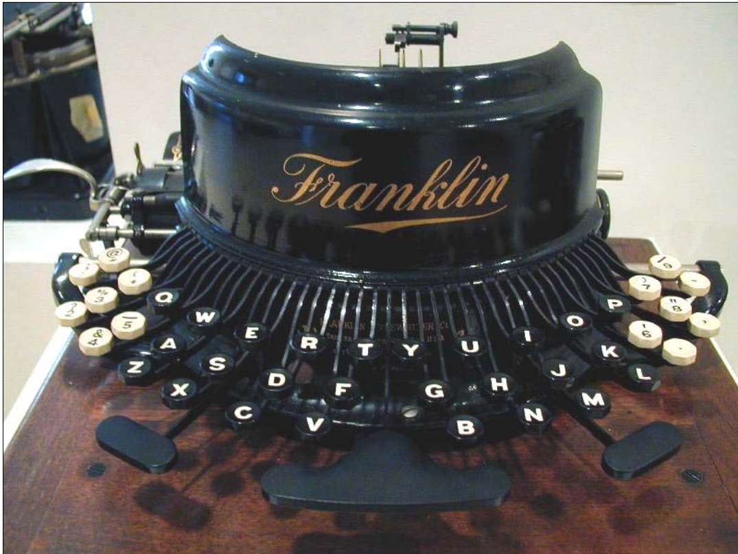
Figure 84. Franklin Typewriter (1891); type bars standing erect, swinging down from the front (downstrike)
