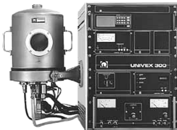
Figure 9.1. LEYBOLD UNIVEX 300 high vacuum device.
