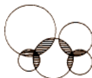
Figure 10.19. Schematic presentation of the overlap of hemispherical centers growing on a monolayer (progressive nucleation).
