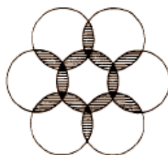
Figure 10.10. Schematic presentation of the overlap of hemispherical centers growing on a monolayer (instantaneous nucleation).
