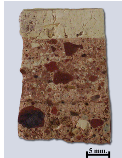
Figure 4.21. Two layers of horasan plaster with single layer of lime plaster taken from upper level (D.I.U.1-D.I.U.2-D.I.U.L)
