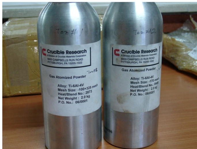
Figure 4.1. Crucible Research Ti6Al4V powders as received.
