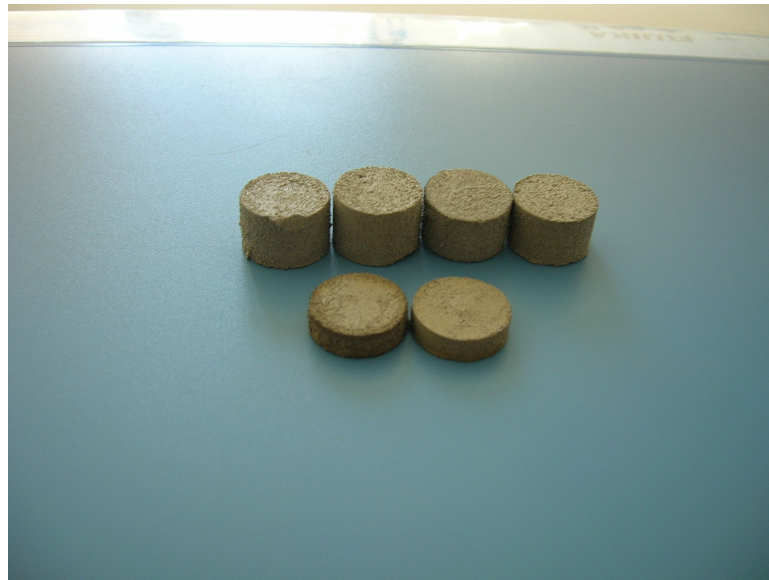
Figure5.4. Cylindrical sintered powder compacts used in the experiments.
