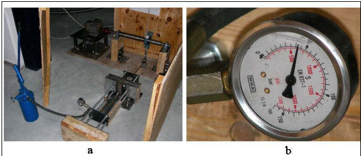
Figure 4.3. (a) The experiment rig for ball bearing testing (b) Adjusted value of the hydraulic jack shown in barometer
