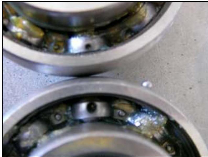
Figure 4.2. The dents on the surface of the ball of bearing
