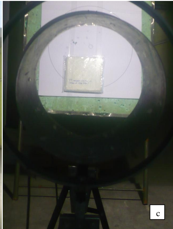
Figure 3.12. Photos showing the ballistic setup at Sarsılmaz Fişek San. A.Ş. a) the test gun, b) the projectile velocity measurement device for 15 m (type III and IV armors), c) the projectile velocity measurement device for 5m (type I, II-A, II and IIIA armors)
