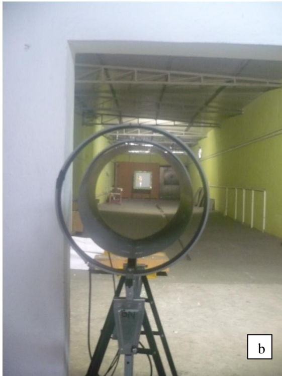
Figure 3.12. Photos showing the ballistic setup at Sarsılmaz Fişek San. A.Ş. a) the test gun, b) the projectile velocity measurement device for 15 m (type III and IV armors), c) the projectile velocity measurement device for 5m (type I, II-A, II and IIIA armors)
