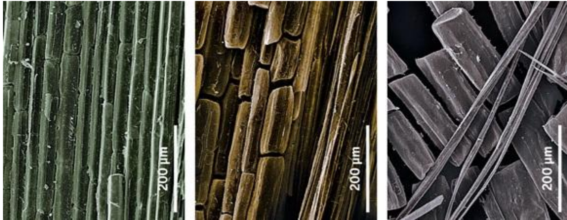
Figure 3.5. The change of corn stover cell walls with acid pretreatment (Source: Brunecky et al. , 2008)
