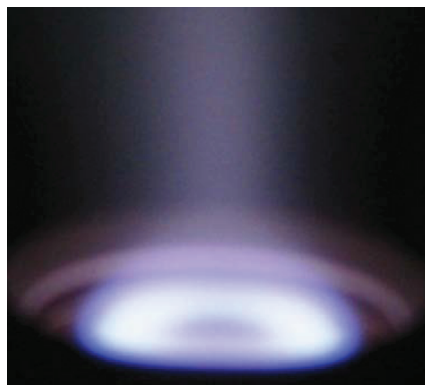
Figure 2.18. Plasma generated during magnetron sputtering
