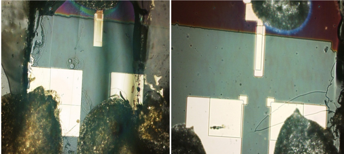
Figure 4.4. Optical image of crystals after gold stripe fabrication by lift off technique
