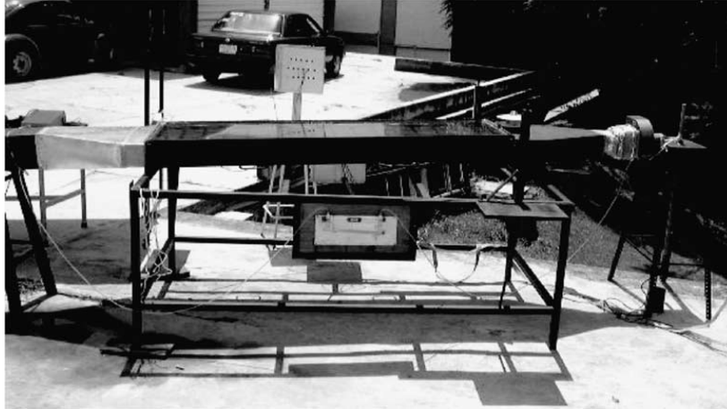
Figure 1.2. A solar air heater collector used in the study of G. Alvarez et al. (Source: G. Alvarez et al., 2010)
