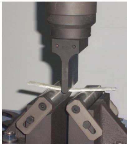
Figure 3.14. Flexural test specimen
