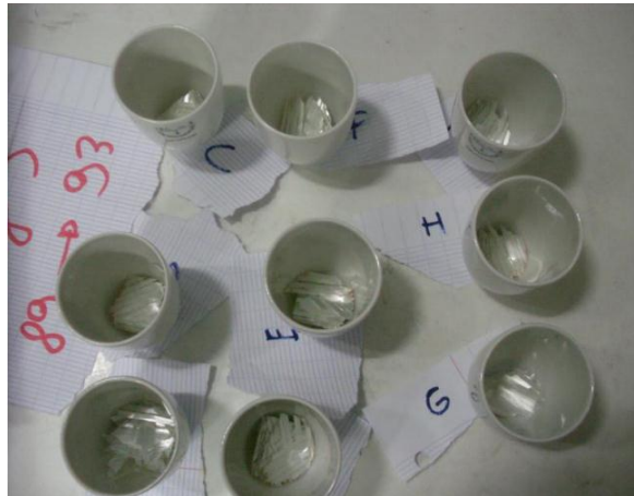
Figure 3.16. Ceramic crucibles and fibers after burn-off process.
