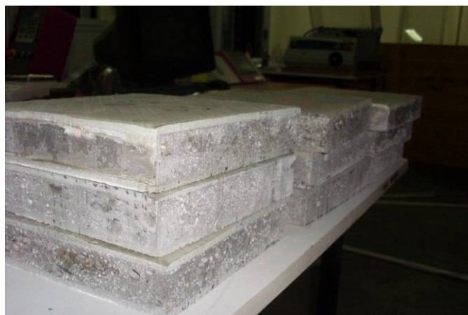
Figure 3.6. Sandwich structures with aluminum foam core.
