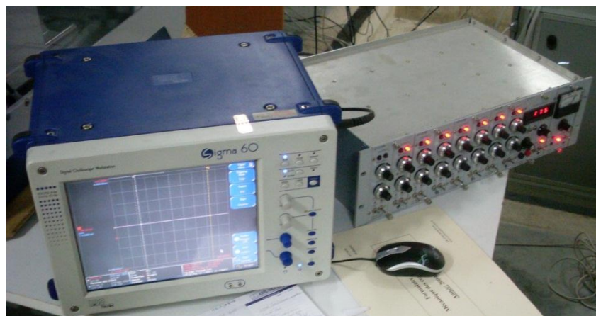
Figure 3.11. Oscilloscope on the left and signal conditioner on the right.
