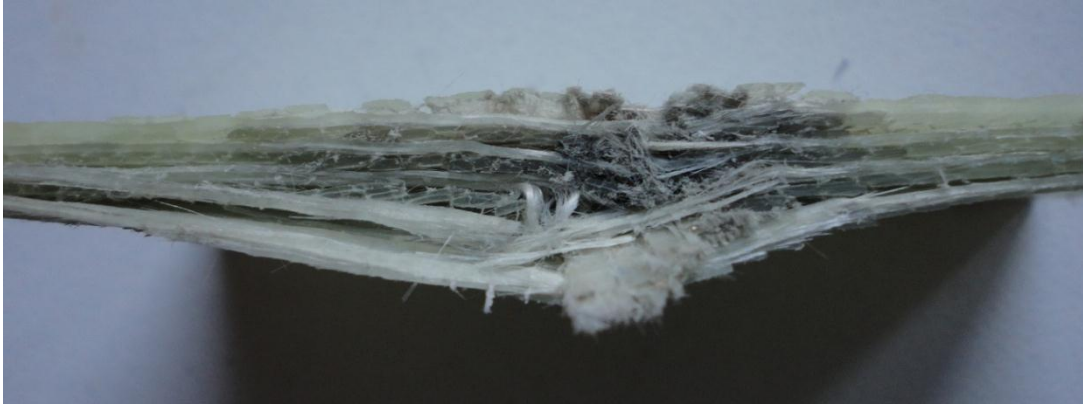
Figure 5.12. 5 mm thick [0^\circ/90^\circ]_s composite sample cross-section for perforation case.
