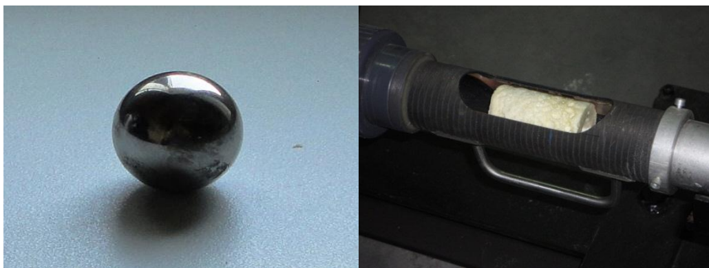
Figure 3.30. (a) Spherical steel projectile and (b) sabot.
