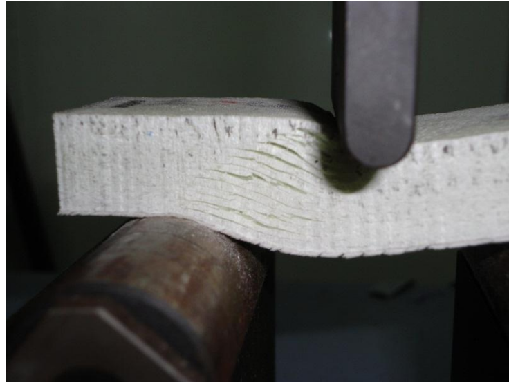
Figure 5.8. Delamination in the short beam test specimen.
