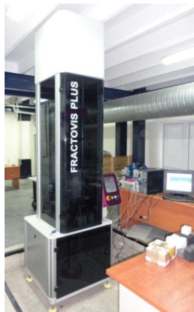
Figure 3.20. FRACTOVIS low velocity impact test equipment.
