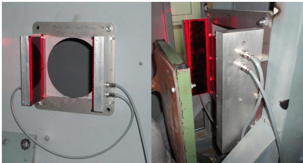
Figure 3.32. Laser barrier (a) before the specimen holder and (b) back of the specimen holder.
