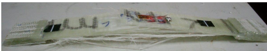
Figure 5.1. The tested tensile test specimens in direction 1.
