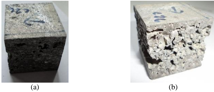
Figure 3.18. Aluminum foam samples (a) 0.11 and (b) 0.15 relative density.
