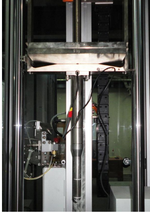
Figure 3.21. Striker holder, weights and the impactor.
