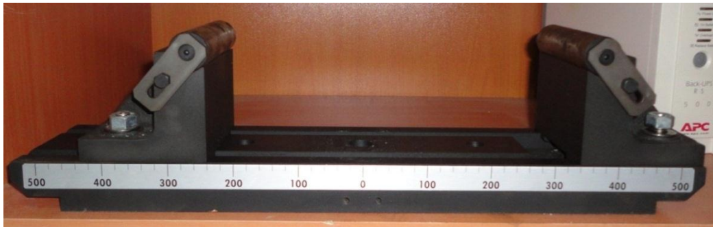
Figure 3.13. Adjustable 3-point bending test fixture.
