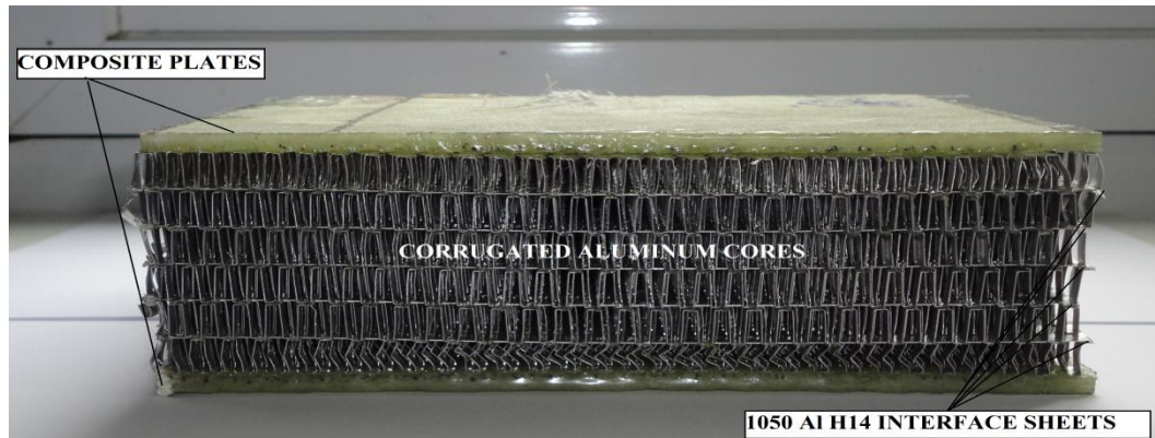
Figure 3.7. Corrugated aluminum core composite sandwich.
