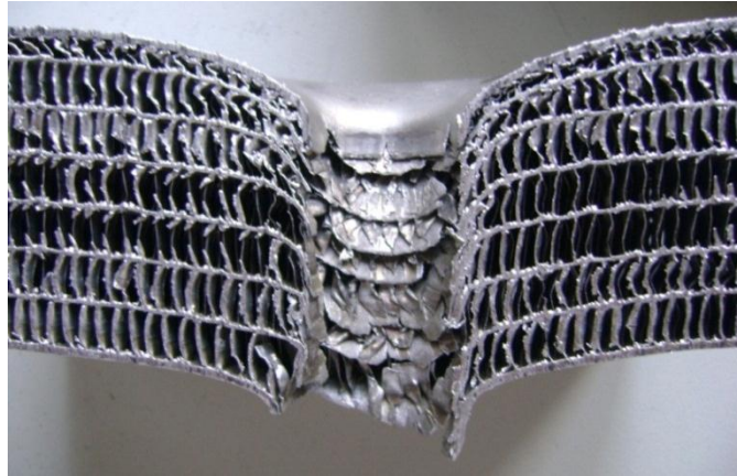
Figure 5.22. Big fin corrugated aluminum core aluminum sandwich cross-sectional view.
