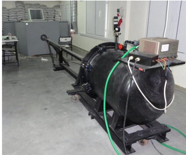
Figure 3.29. Overview of the projectile impact test setup.
