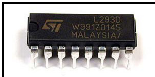
Figure 3.11. L293, H – bridge (Source: toko-robot.com)
