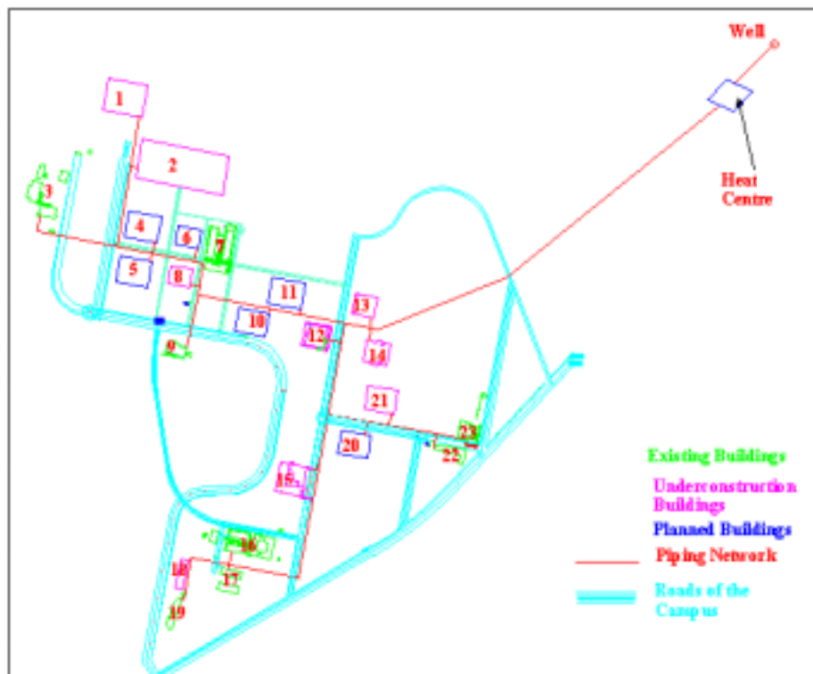
Figure 6.19: Alternative 2 for district heating piping network.
