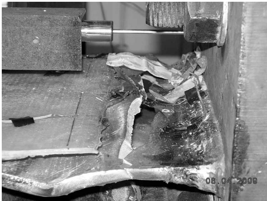
Figure 4.14. HE400AA GFRP2 Beam Top Flange Fracture at 0.046 rad of Rotation
