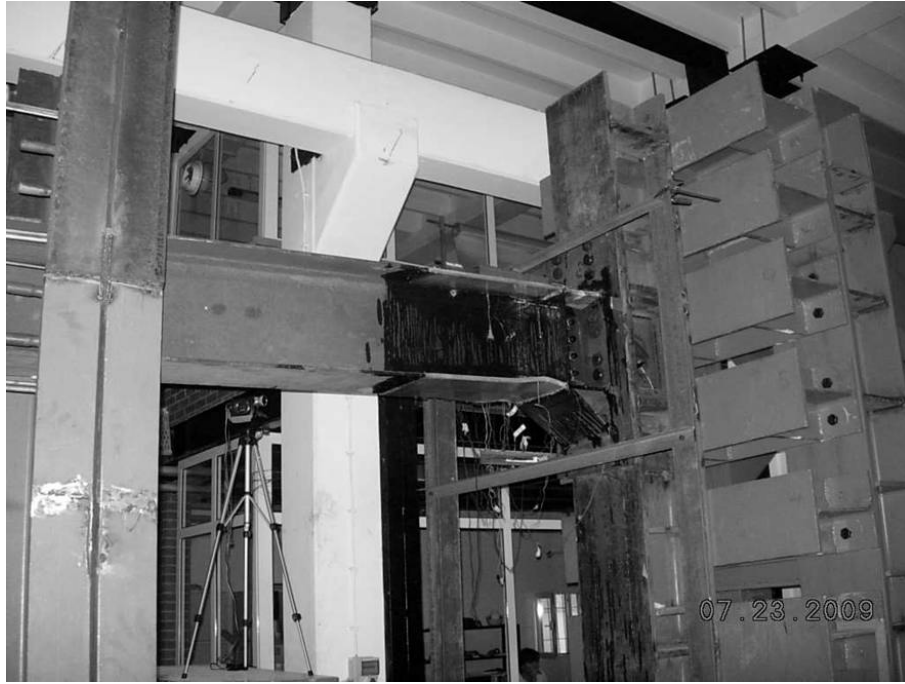
Figure 4.19. HE400AA GFRP3 Beam Bottom Flange at 0.043 rad of Rotation
