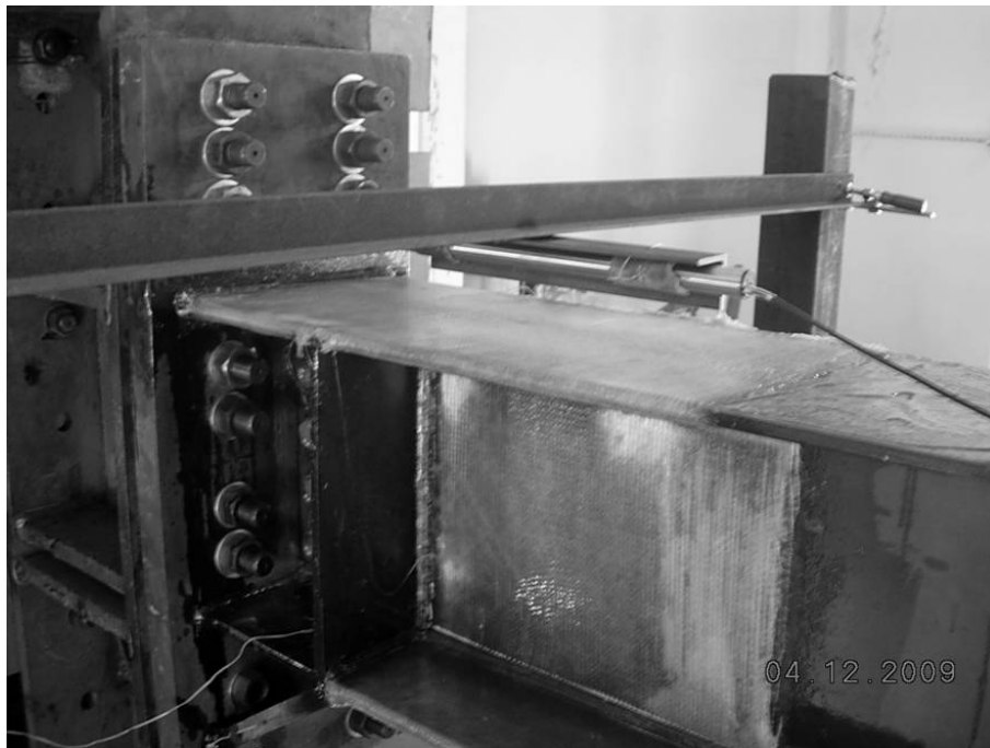
Figure 3.17. HE400AA GFRP1 Beam
