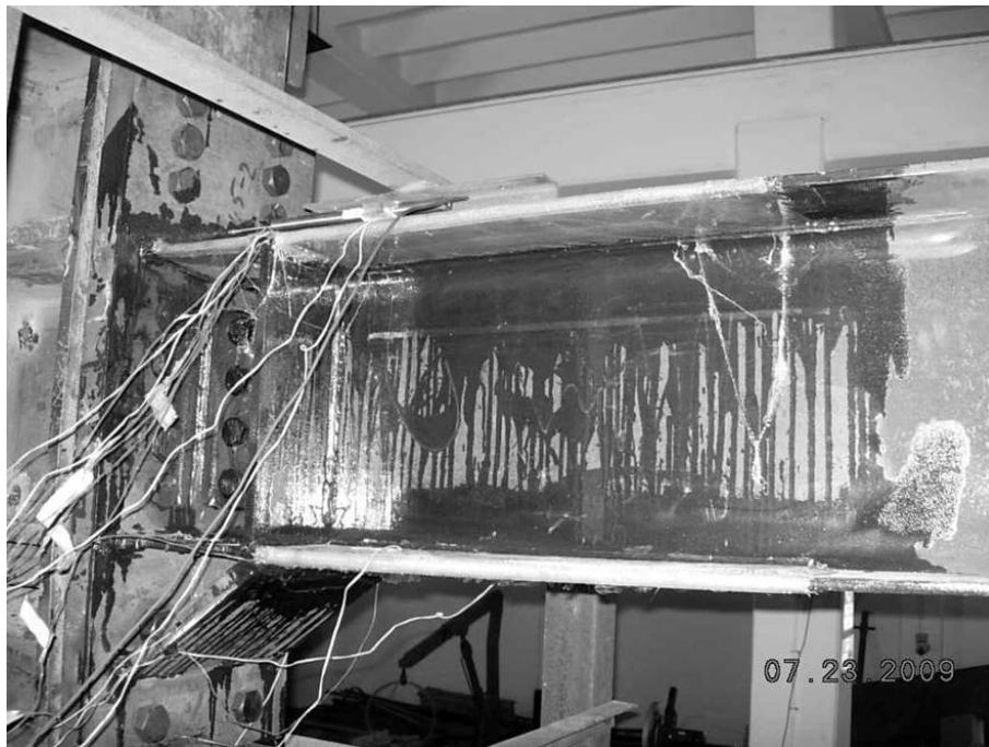
Figure 3.21. HE400AA GFRP3 Beam
