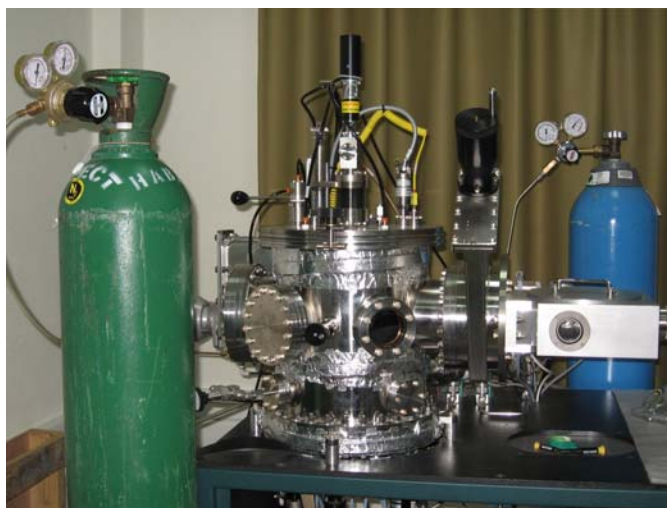
Figure 3.2. ATC Orion 5 UHV Magnetron Sputtering System
