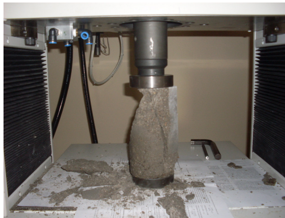
Figure 4.20. Universal Test Machine used (at IYTE-MAM) for the Unconfined Compression Tests conducted on the prepared C-PSL Test Specimens-Shearing Failure, Close-up View
