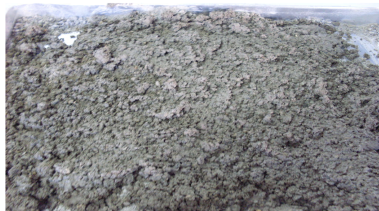
Figure 4.13. Thoroughly Mixing the Sand-Cement Mixture
