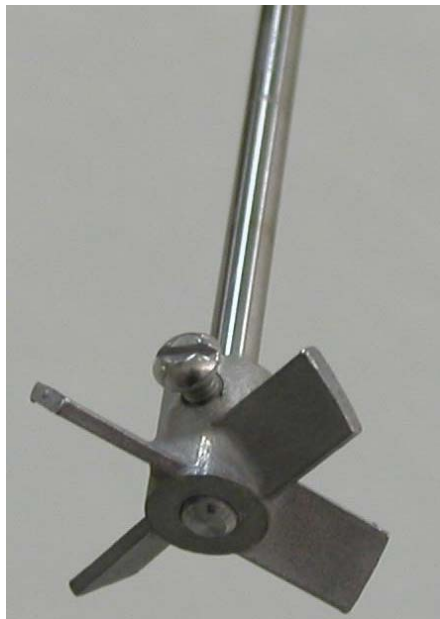
Figure 4.3. Photograph of impeller used in the stainless steel reactor.
