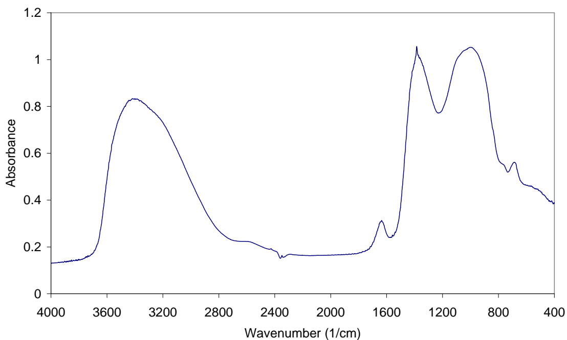
Figure 5.100. FTIR spectrum of freeze dried zinc borate produced from borax and zinc nitrate (S-21).
