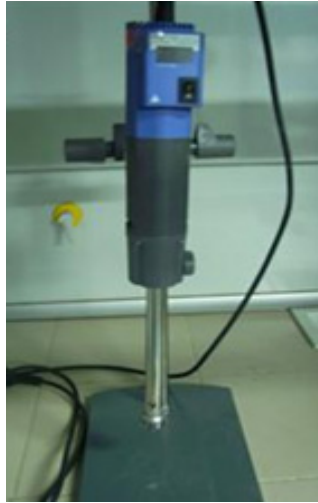
Figure 6.1. Ultra-Turrax mechanical disperser.
