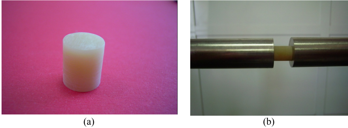
Figure 6.9. (a) SHPB compression test specimen and (b) the specimen inserted in between the bars.
