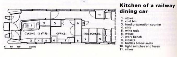
Figure 3.16. The diagram comparing the dimensions of kitchens and kitchen of a railway dining car, 1920-25? (Source: Teige 1932)
