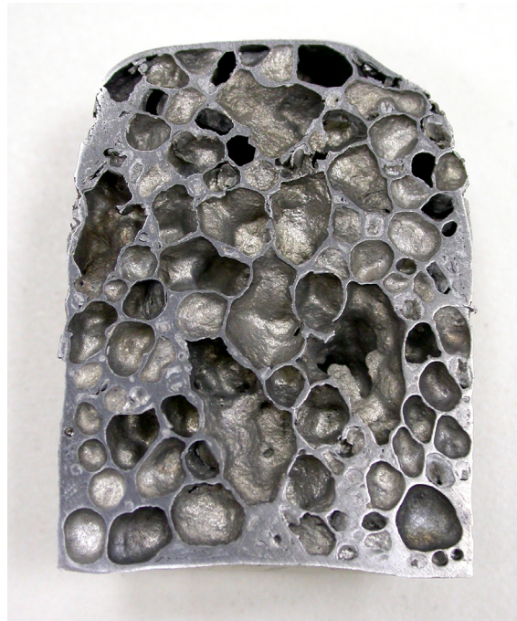
Figure 4.1. Cross-section of aluminum foam showing thin cell walls, thick cell edges and dense metal layer at the bottom section.
