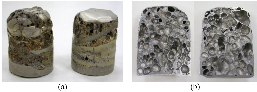
Figure 6.3. Pictures of the foams with 0.6 wt% \text{TiH}_2 blowing agent addition (at maximum expansion); (a) uncut and (b) cross-section.
