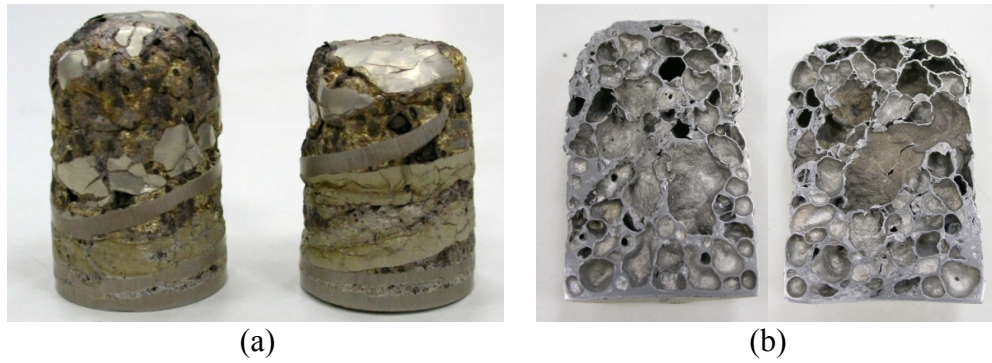
Figure 6.5. Pictures of the foams with 1.0 wt% TiH 2 blowing agent addition (at maximum expansion); (a) uncut and (b) cross-section.
