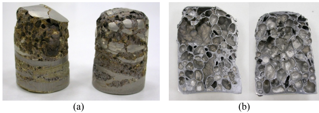
Figure 6.4. Pictures of the foams with 0.8 wt% \text{TiH}_2 blowing agent addition (at maximum expansion); (a) uncut and (b) cross-section.
