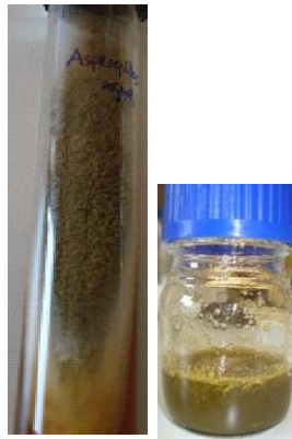
Figure 5.2.(a) Spores grown on molasses agar slants,(b)spore suspension used for inoculation.
