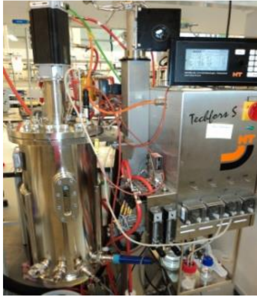
Figure 5.5. 20 l scale Techfors, INFORS bioreactor
