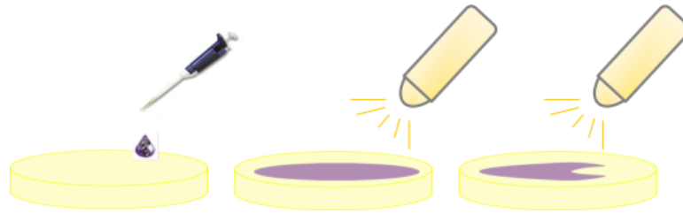
Figure 6. 4 Schematic diagram of the drop size DNA nitrogen flow regime drying procedure
