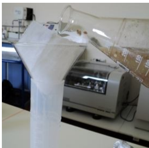
Figure 5.3. Filtration of the flask content through the cheese cloth
