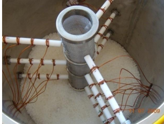
Figure 7.5. An inside view of the designed adsorbent bed and locations of the thermocouples
