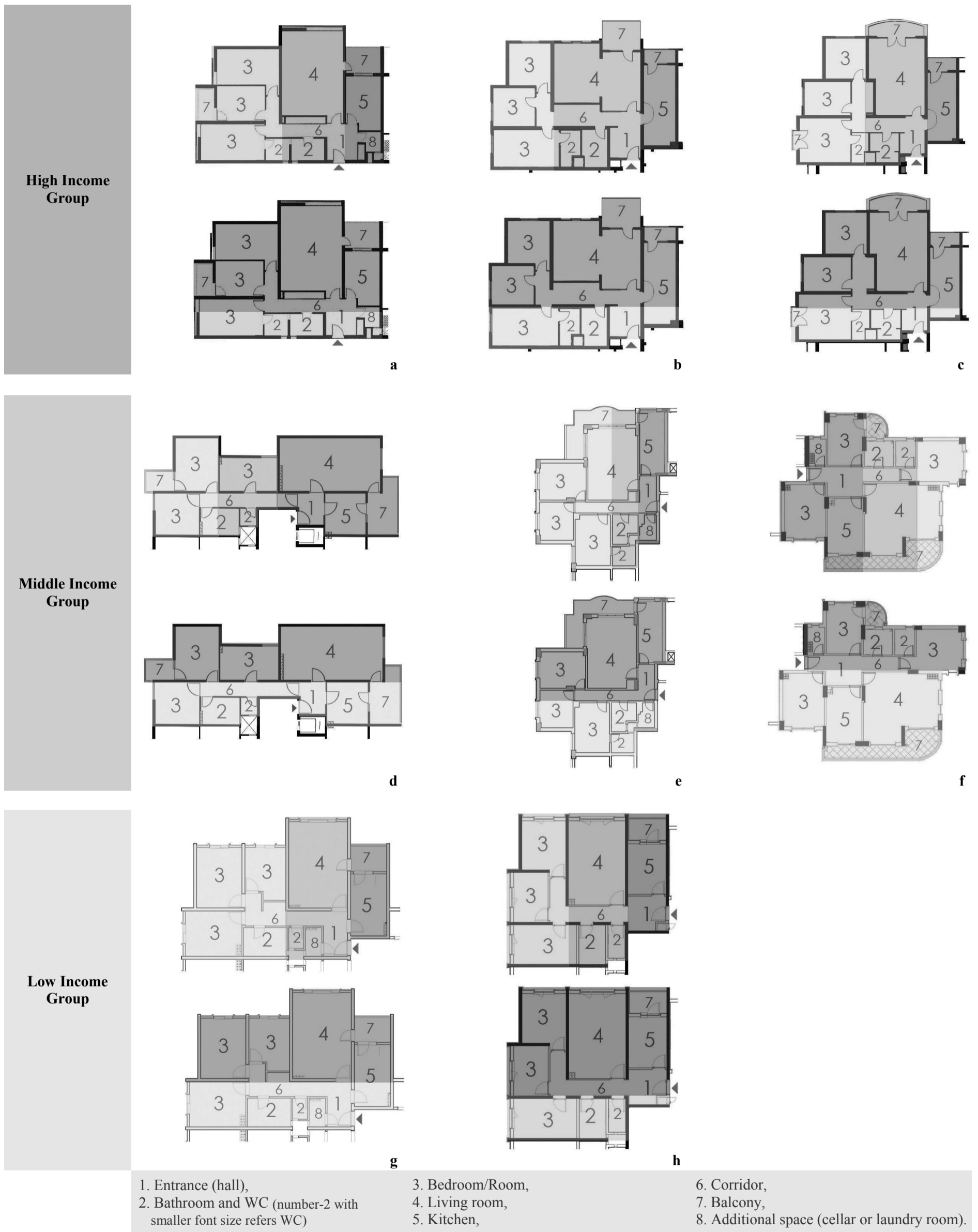
Figure 6.4. Linear readings of the spatial alignments of 3+1 units in six cases: a. Albayrak Mavişehir Housing: Above: latitudinal division, Below: longitudinal division; b. Soyak Mavişehir Housing: Above: latitudinal division of B-type, Below: longitudinal division of B-type; c. Soyak Mavişehir Housing: Above: latitudinal division of C-type, Below: longitudinal division of C-type; d. Mimkent 1 Mass-Housing: Above: latitudinal division, Below: longitudinal division; e. Ege-Koop Körfez Houses: Above: latitudinal division of B-type, Below: longitudinal division of B-type; f. Ege-Koop Körfez Houses: Above: latitudinal division of C-type, Below: longitudinal division of C-type; g. Narbel Mass-Housing: Above: latitudinal division, Below: longitudinal division; h. TOKI Buca Mass-Housing: Above: latitudinal division, Below: longitudinal division (Sources: Analyses were prepared by İpek Ek regarding the plan drawings taken from the following sources: a. Tamer Başbuğ's archive; b., c. Soyak 2009; d. Archive of Karabağlar Municipality; e., f. Ege-Koop's archive; g. Demirer Group's archive; h. TOKI's archive)
