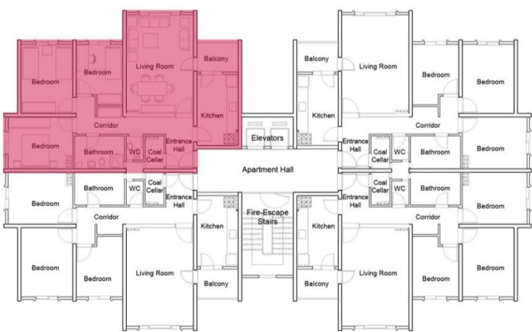
Figure 6.2. Comparison of the floor plans of six cases (units with red refer the ones having 3+1 plan-schemes examined in the research): a. Floor plan of Albayrak Mavişehir Housing; b. B-type floor plan of Soyak Mavişehir Housing; c. C-type floor plan of Soyak Mavişehir Housing; d. Floor plan of Mimkent 1 Mass-Housing; e. B-type floor plan of Ege-Koop Körfez Houses; f. C-type floor plan of Ege-Koop Körfez Houses; g. C-type floor plan of Narbel Mass-Housing; h. C-type floor plan of TOKI Buca Mass-Housing (Sources: a. Tamer Başbuğ's archive; b., c. Soyak 2009; d. Archive of Karabağlar Municipality; e., f. Ege-Koop's archive; g. Demirer Group's archive; h. TOKI's archive)
