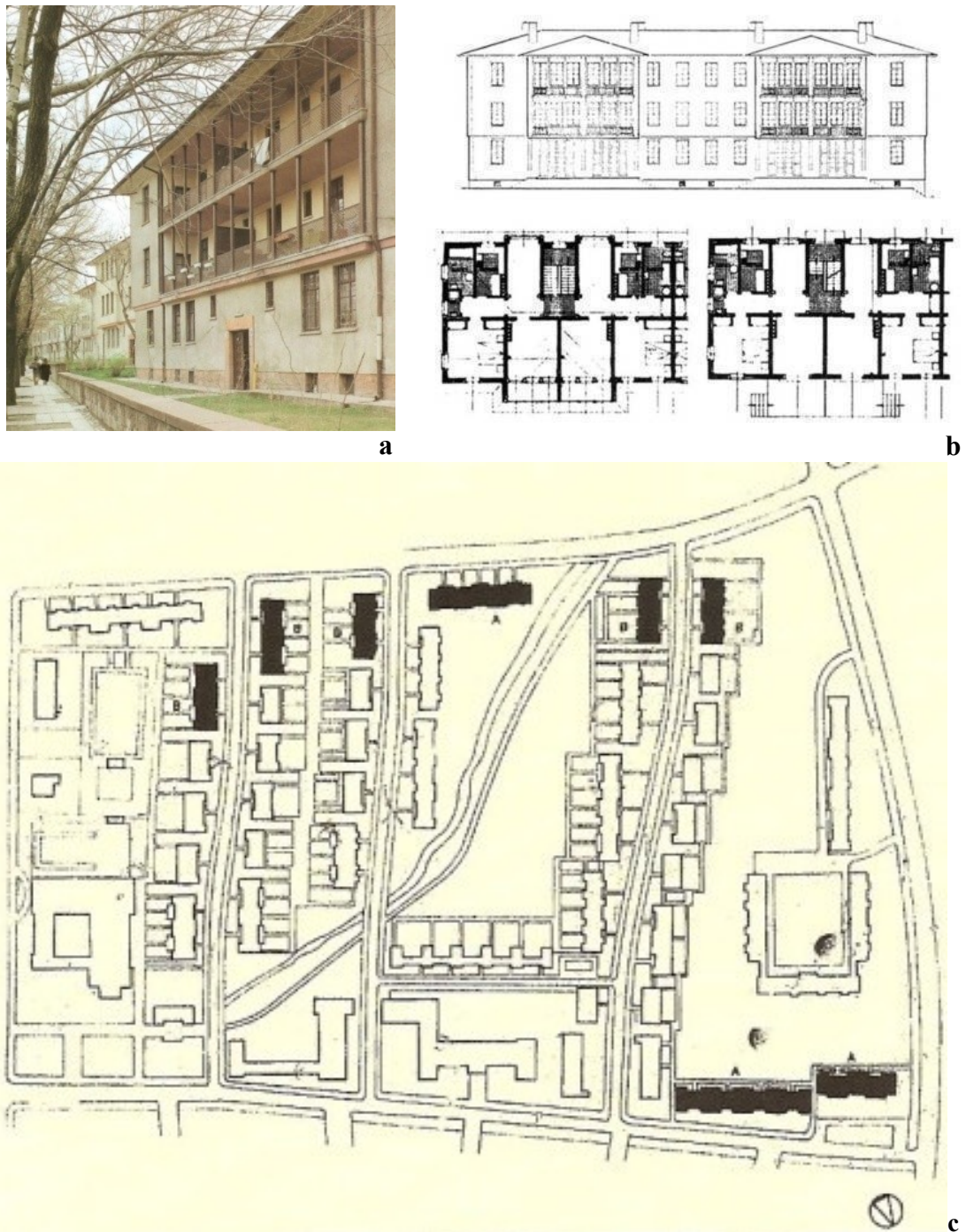
Figure 2.9. Saraçoğlu District designed by Paul Bonatz, Ankara, 1946: a. Outside view; b. Elevation and floor plan; c. Site plan (Sources: a. Sey 1999, 295; b. Architecture Museum 2011b; c. Tapan 1996, 367)
