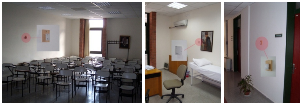
Figure 37. Data loggers in different spaces (classroom, office, and corridor)
