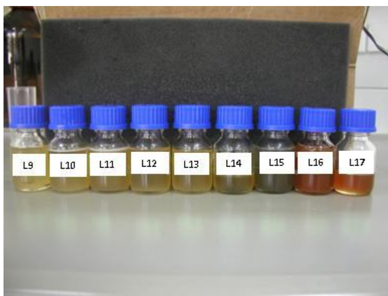
Figure 7.81. The photographs of the prepared lubricants. Mineral oils with sorbitan monostearate and L9: zinc borate produced by coordination homogeneous precipitation, mixed for 6 h. L10: zinc borate produced by coordination homogeneous precipitation, mixed for 15 h, L11: zinc borate produced by coordination homogeneous precipitation, mixed for 12 h., L12: 0.00005 g sorbitan monostearate and zinc borate mixed for 12 h. L13: mineral oil, 0.1 g sorbitan monostearate and zinc borate, L14: precipitate obtained by inverse emulsion having 30% propanol-2, L15: clinoptilolite rich mineral, L16: inverse emulsion of which water was removed by water, L17: inverse emulsion of which water was removed by clinoptilolite rich mineral.
