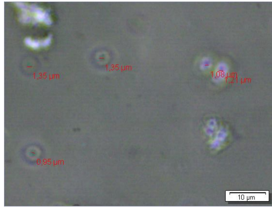
Figure 7.73. The microphotograph of the lubricant containing surfactant and clinoptilolite rich mineral (The microphotograph was taken by Olympus BX60M microscope).
