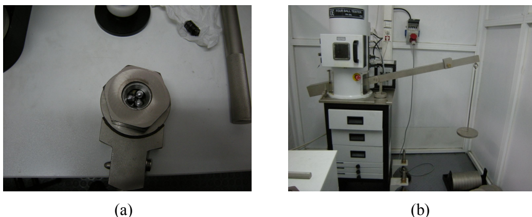
Figure 6.3. a) Fixed balls of four-ball wear tester b) Whole machine of four-ball tester.
