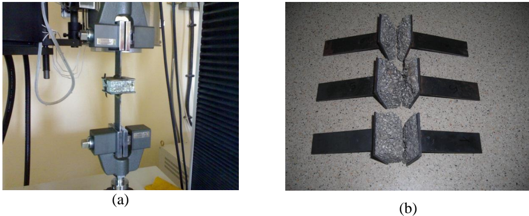
Figure 5.9. Al foam samples subjected to tensile testing: (a) 20 mm Al foam during tension test, (b) Test coupons after test tension test.
