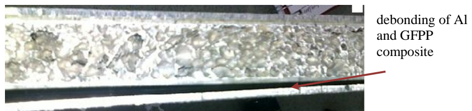
Figure 5.47. Side view of the sandwich test panel with 20 mm Al foam after loading up to the end of 2 nd region with stress vs. central deflection plot.
