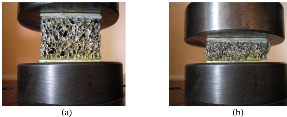
Figure 4.17. The Al sheet/GFPP/Al foam sandwich with 30 mm Al foam thickness (a) before loading (b) at 50% deformation.
