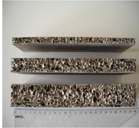
Figure 4.2. As-received ALULIGHT™-AFS Al foam panels with 8, 20 and 30 mm thickness.
