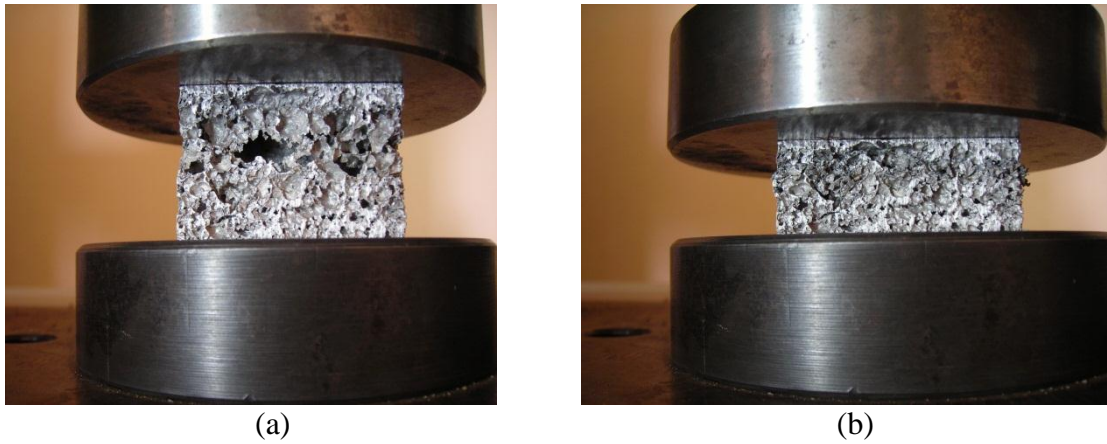
Figure 4.9. Compression characteristics of 30 mm Al foam: (a) before loading, (b) at 50% deformation
