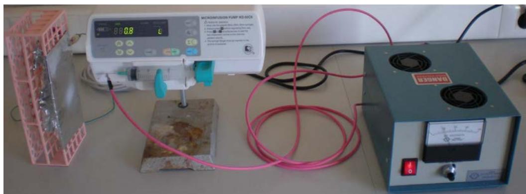
Figure 3.4. Experimental set-up used in electrospinning process
