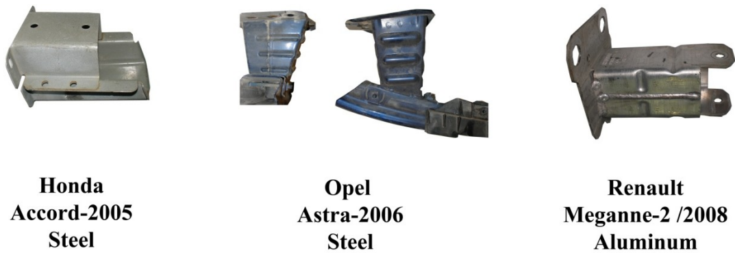
Figure 1. 4. Commercial crash boxes in various geometries.
