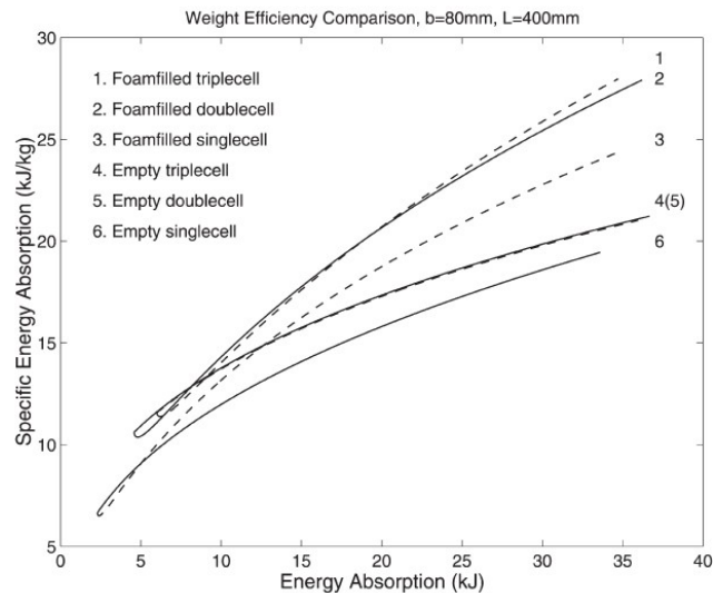
Figure 3.27. SEA values of empty and foam filled single, double and triplecell square Al sections (Source: Chen and Wierzbicki 2001)
