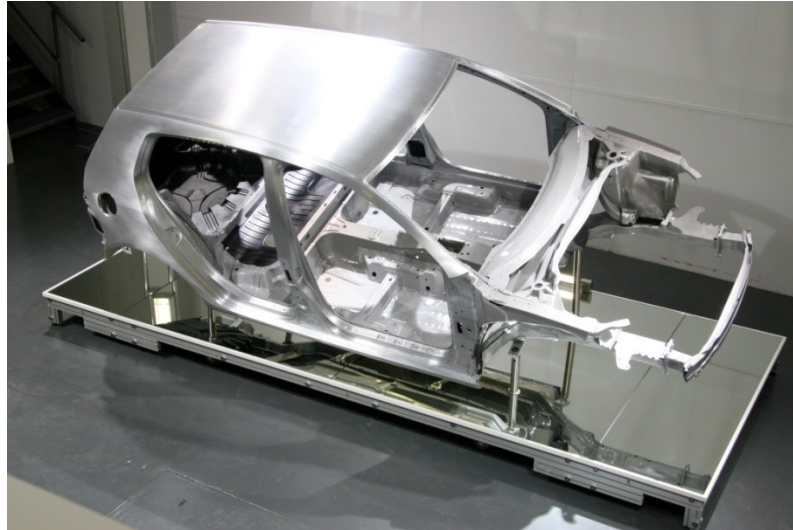
Figure 1. 1. The body in white structure of Super Light Car, with approximately 32% reduction in weight,(Source: Duwe and Kopp 2009).
