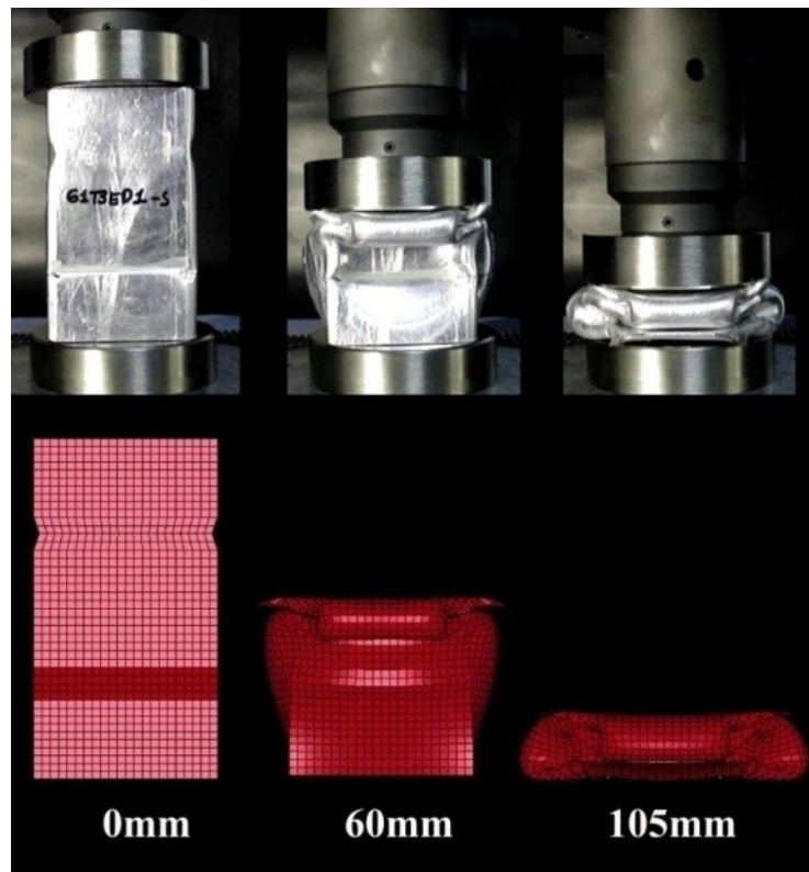
Figure 7.4. Sequential deformation photos of empty crash box without montage parts, t=3 mm (G1T3E).
