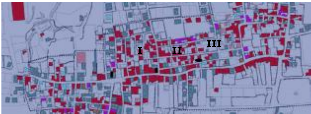
Figure 4.3. Measured Houses shown on the map of Alaçatı Kemalpaşa Street. (The house represented with I is cross-ventilated, the house represented with II is single side-ventilated sofa example, and the point represented with III is where the rooftop measurements are taken)
