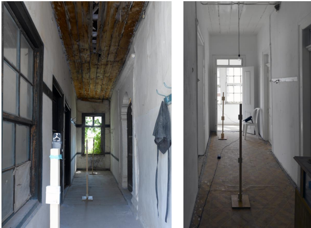
Figure 4.8. Measured house I_ cross ventilated sofa Measured house II_ single-side ventilated sofa
