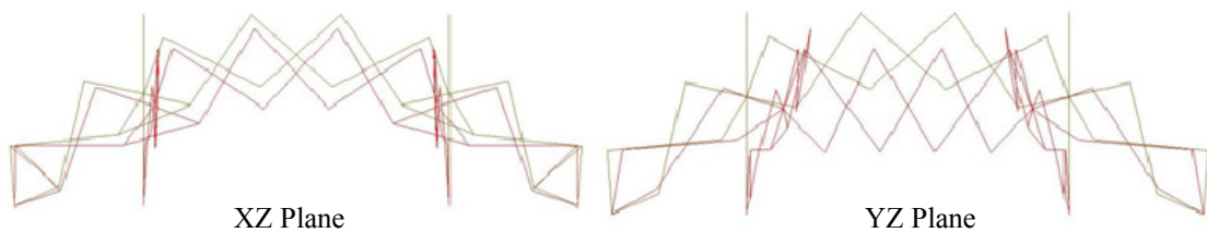
Figure 91. Undeformed (black) and deformed (red) shapes of the cross vault shaped structure
