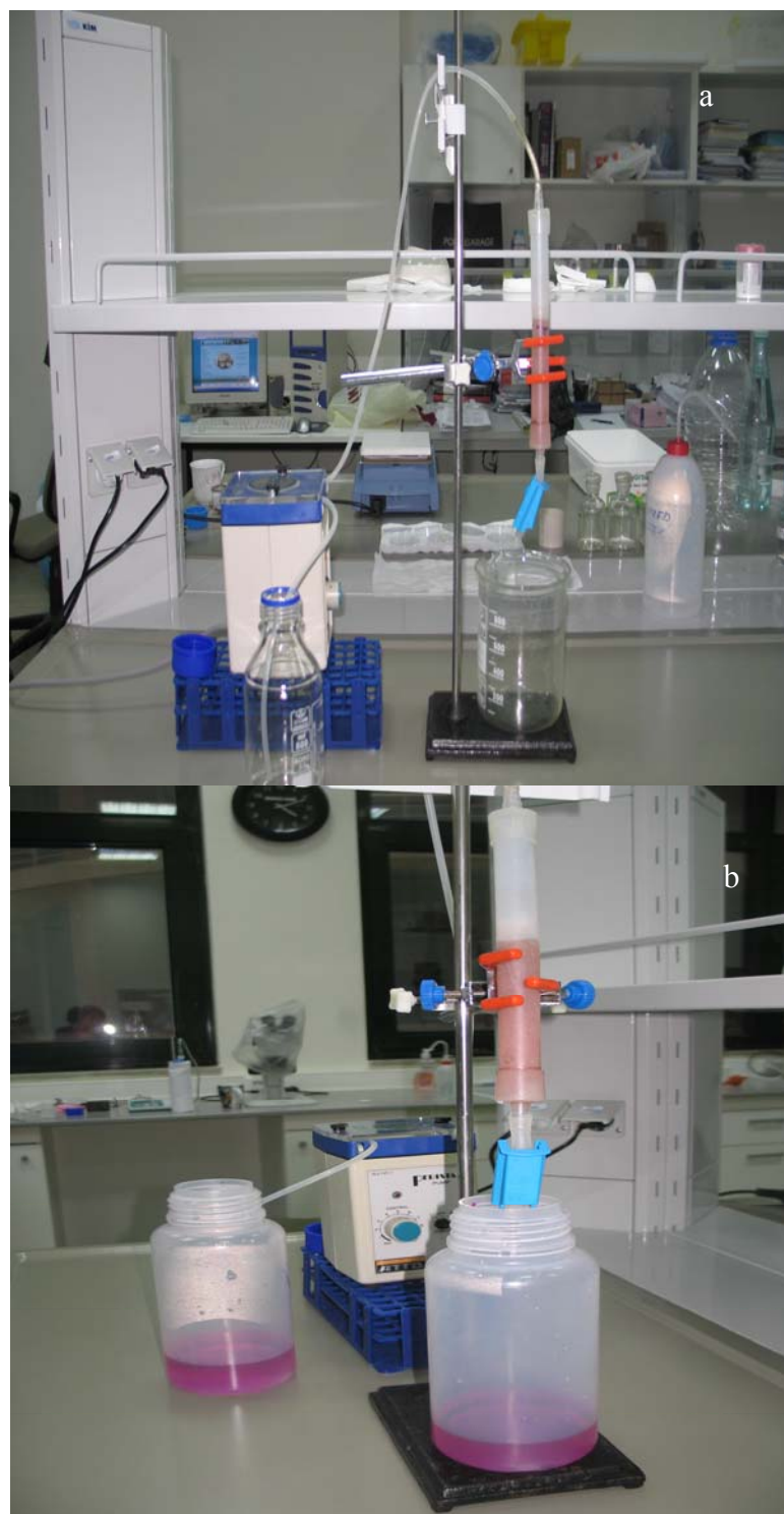
Figure A.1. Cation exchange column chromatography system used to purify Arsenazo III dye a. front view, b. side view.
