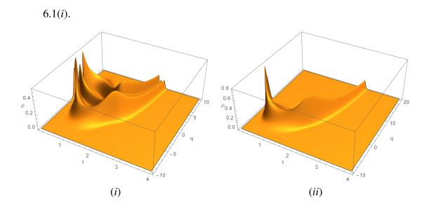
Figure 6.3. Laguerre type generalized oscillator, when  $D(t) = (t - 2)L_2(t)$ ,  $E(t) = (1 - t)L_2(t)e^t$ . (*i*) Probability density  $\rho_2^{1,1}(q, t) = |\Psi_2^{1,1}(q, t)|^2$ , n = r = 1, and k = 2. (*ii*) Probability density  $\rho_{\alpha}^{1,1}(q, t) = |\Psi_{\alpha}^{1,1}(q, t)|^2$  in coherent states for  $\alpha = 1/\sqrt{2} + i(1/\sqrt{2})$ , n = r = 1.
