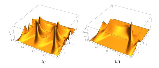
Figure 7.1. Legendre type generalized oscillator, when  $D(t) = tP_2(t)$ ,  $E(t) = -P_2(t)/6$ , F(t) = 0. (*i*) Probability density  $\rho_2^{2,2}(q,t) = |\Psi_2^{2,2}(q,t)|^2$ . (*ii*) Probability density  $\rho_\alpha^{2,2}(q,t) = |\Phi_\alpha^{2,2}(q,t)|^2$  in coherent states for  $\alpha = 1/\sqrt{2} + i(1/\sqrt{2})$ .
