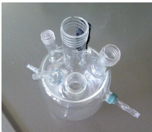
Figure 3.3. 5-neck jacketed reactor
