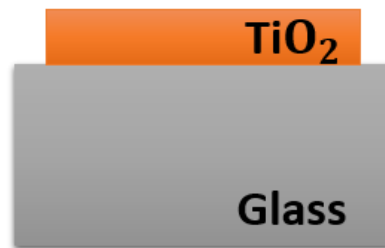
Figure 5.1. The structure of Glass + TiO 2 (with 250nm thickness)
