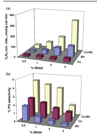
Fig. 7 Activity and selectivity of Cu, Mn and Cu-Mn/α-Al<sub>2</sub>O<sub>3</sub>
