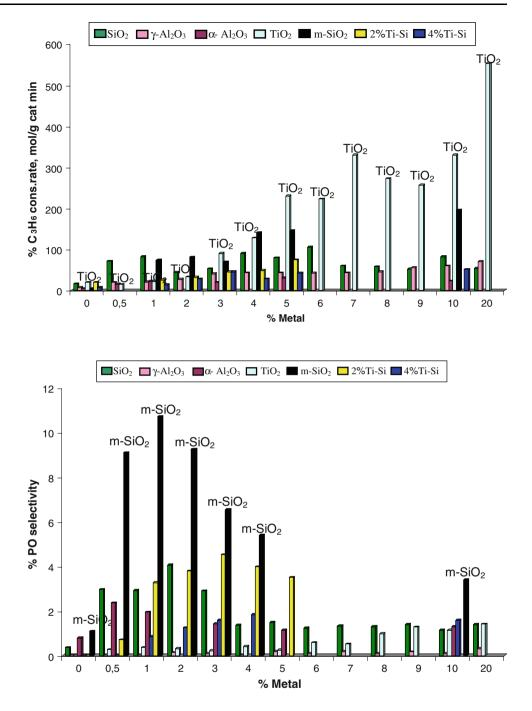
Fig. 3 PO selectivity of supported Cu catalysts SiO<sub>2</sub>,  $\gamma$ -Al<sub>2</sub>O<sub>3</sub>,  $\alpha$ -Al<sub>2</sub>O<sub>3</sub> TiO<sub>2</sub>, m-SiO<sub>2</sub>, 2%Ti–Si, 4%Ti–Si
