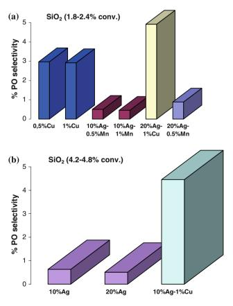
Fig. 6 PO selectivity of Ag&Cu and Ag&Mn/SiO<sub>2</sub> catalysts at the same conversion values (a) 1.8-2.4% and (b) 4.2-4.8% conversion
