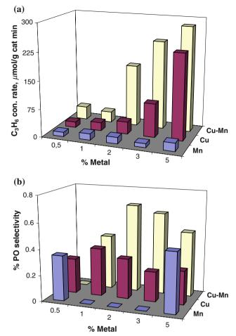
Fig. 8 Activity and selectivity of Cu, Mn and Cu-Mn/TiO<sub>2</sub> catalysts
