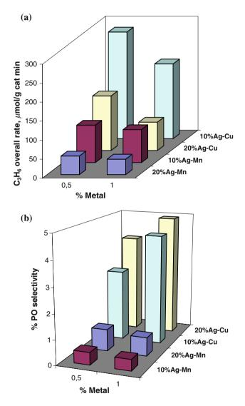
Fig. 5 Activity and selectivity of Ag&Cu and Ag&Mn/SiO<sub>2</sub> catalysts
