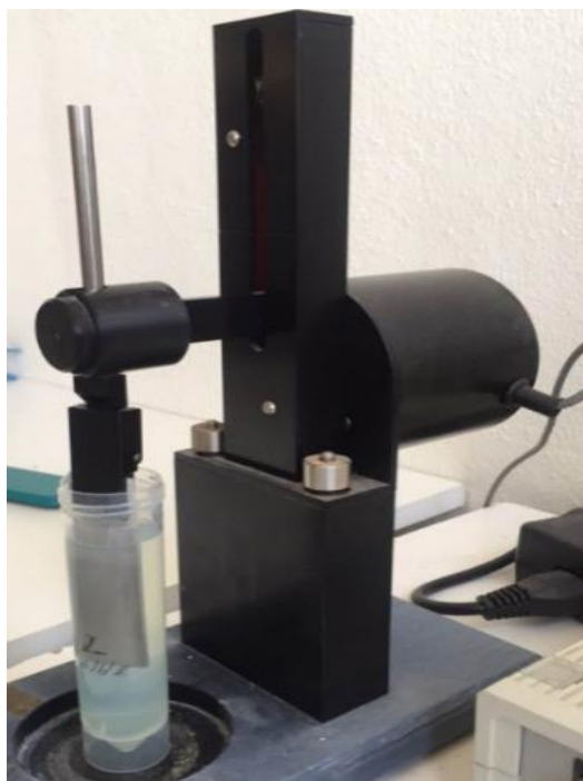
Figure 3.1. Image of dip-coating process with Nima Dip-coater equipment
