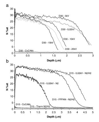
Fig. 5. GDOES nitrogen atomic concentration profiles obtained on a) on D30-CoCrMo nitrided in pure  $N_2$  b) on nitrided D15-CoCrMo.
