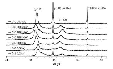
Fig. 2. X-ray diffraction patterns obtained on the D30 samples and on the D15-0.02 kV-N2 sample for comparison.
