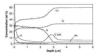
Fig. 4. GDOES atomic concentration profiles obtained on PBII nitrided D30-CoCrMo (5 kV – 400  $^\circ\text{C}$  – N2).
