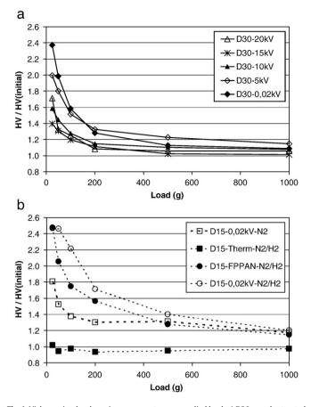
**Fig. 1.** Vickers microhardness improvement versus applied load. a) D30 samples treated by PBII in N2 plasma; b) D15 samples treated without plasma in N2/H2, with N2/H2 plasma at floating potential (FPPAN) or with N2/H2 and N2 at 0.02 kV. The HV values were obtained with at least 4 different measurements, with accuracy of about 20% (25 g), 15% (50 g) or less than 10% (100 g to 1000 g).
