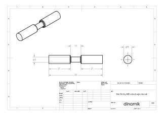
Figure 5. Dimensions of dynamic test specimens
