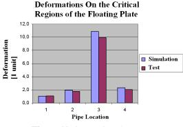
Figure 11. Comparison between field test and simulation
