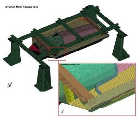
Figure 8. FEA model of Fixture
