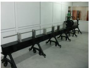
Figure 3. Split-Hopkinson Pressure Bar apparatus
