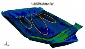
Figure 12. Stress concentration on the V-hull
