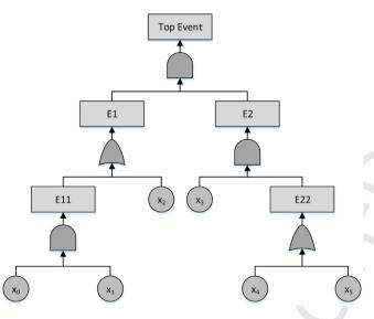
Fig. 7. Fault tree model used as a benchmark [42].
