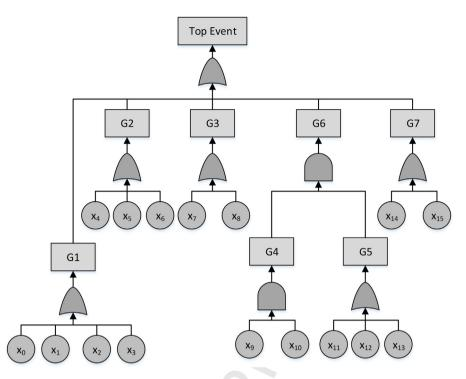
Fig. 9. Fault tree model derived from a software architecture (FT1-SC14) [22].
