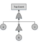
**Fig. 5.** Example non-coherent fault tree model ( $p_a = p_b = p_c = 0.1$ ).
