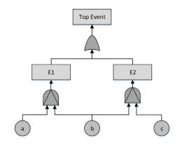
**Fig. 6.** An example dynamic fault tree model ( $p_a = 0.05$ ,  $p_b = 0.06$ ,  $p_c = 0.01$ ).
