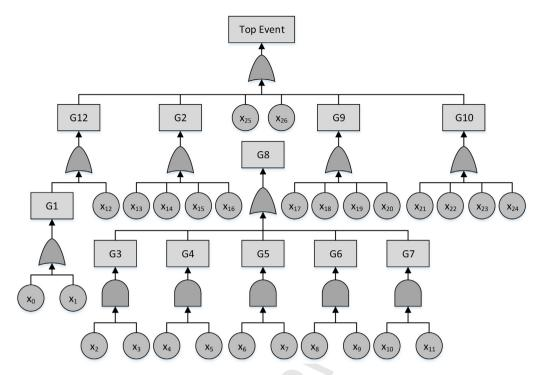
Fig. 11. Fault tree model derived from a software architecture (SC0-10) [22].
