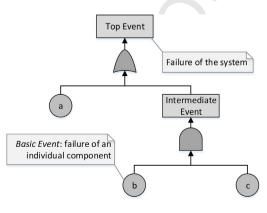
Fig. 1. An example fault tree model.
