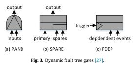
and one or more spare inputs. If the failure of primary input occurs, it is replaced by one of the spare inputs. The primary and all the spare input events must take place (all the corresponding components must fail) for the output event of the SPARE gate to occur. A spare input can be shared among multiple SPARE gates. In this case, if a spare is already utilized by any of the SPARE gates, it is considered to be unavailable (failed) for the other SPARE gates that share it.
