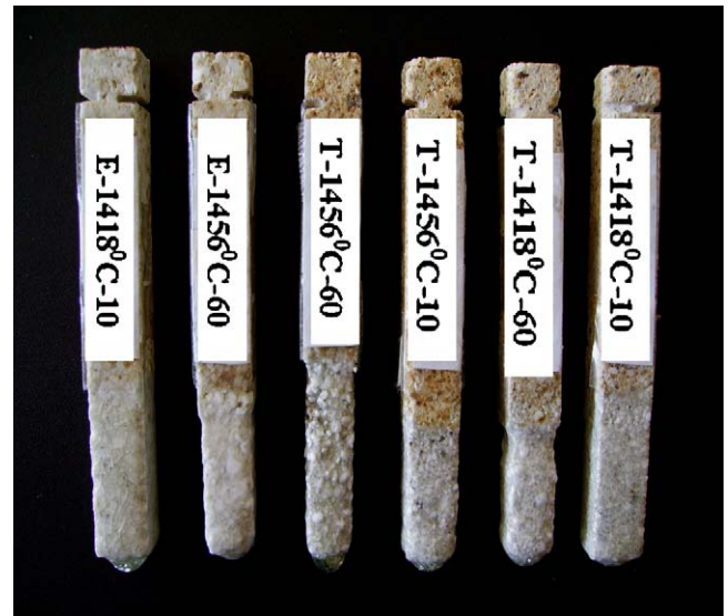
Fig. 13. A photograph of the corroded refractory bricks after dynamic corrosion tests. The following code was used indicate sample exposure conditions: E-1418 °C-10: E refractory specimen was tested at 1418 °C during 10 min.
