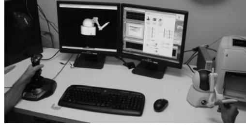
Fig. 6. Experimental setup for commercial joystick as the master and Phantom Omni Device as the slave
