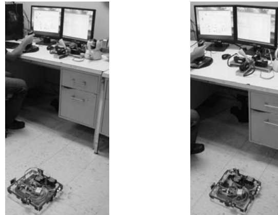
Fig. 10. Experimental setup for the master joystick and the holonomic mobile platform
