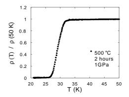
Fig. 4. Temperature dependence of the resistivity of the produced MgB<sub>2</sub>.
