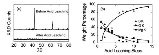
Fig. 1. (a) XRD patterns, before and after acid leaching of the powders obtained after the reaction of  $B_2O_3$  and Mg at 800 °C (b) Variation of the B purity with respect to the number of acid leaching steps.
