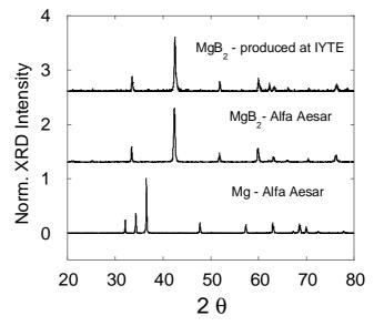
Fig. 2. Normalized XRD patterns of the produced MgB<sub>2</sub>.
