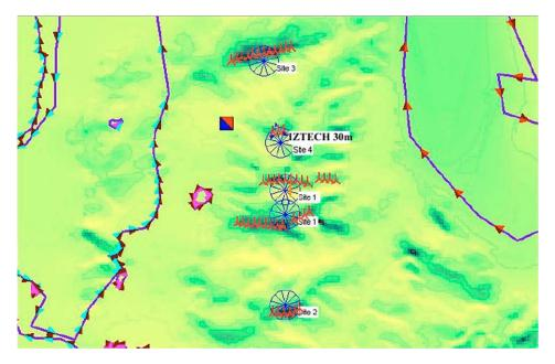
Fig. 4. Micrositting of  $600\ kW$  turbines on the campus area.
