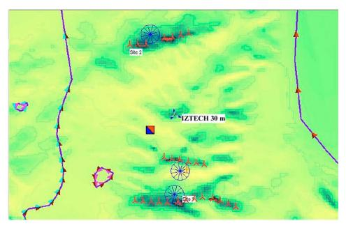
Fig. 5. Micrositting of 1500 kW turbines on the campus area.
