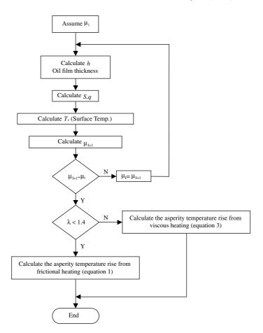
Fig. 1. Flow chart of temperature rise calculation, where viscosity constant at maximum surface.
