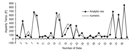
Fig. 3. Predicted analytical results of aspererity temperature given by Eqs. (2) and (3) depend on lubrication condition and predicted numerical results of asperity temperature.
