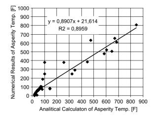
Fig. 4. Predicted numerical results vs. analytical results of asperity temperatures and  $R^2$  value.
