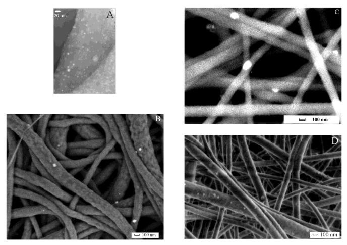
**Figure 4.** Electron microspcope images of PAN-AA fibers with generated Pd nanoparticles: (a) sample A, (b) sample B, (c) sample C, and (d) sample D. Sample A is magnified 300K times and the others 50K times.
