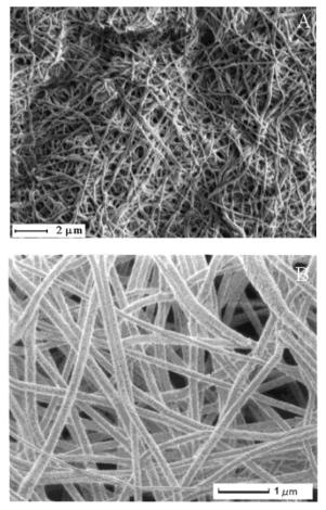
**Figure 2.** Electron microspcope images of nanofibers electrospun from 8 wt % PAN with (a) 5.4% mol AA and (b) 8.1% mol AA under 1.8 kV/cm.
