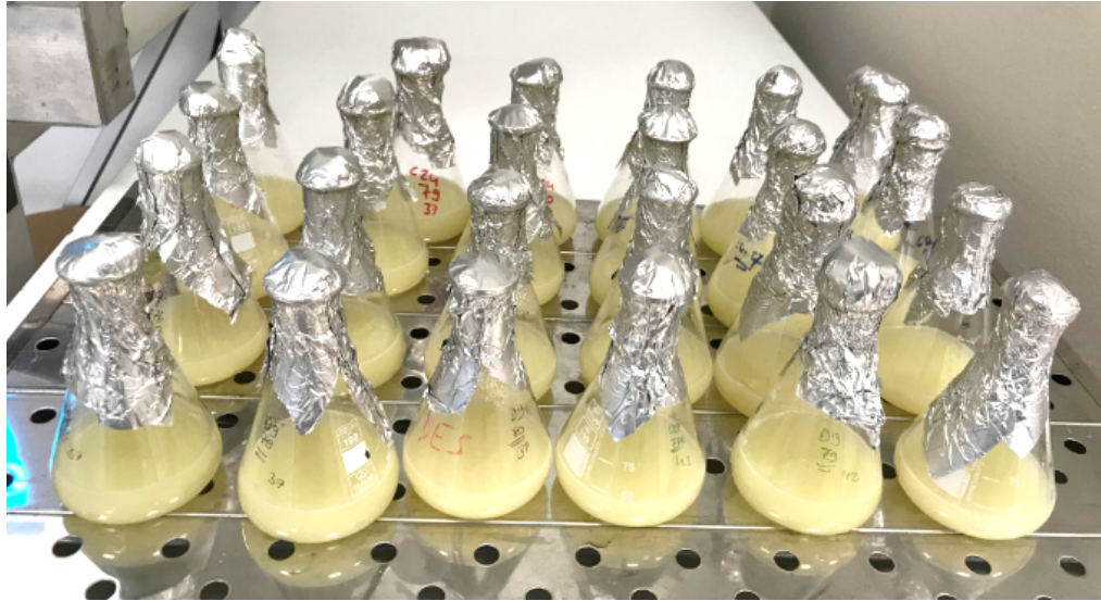
Figure A.21. Fermented whey sample. Co-culture fermentation; L. plantarum or L. lactis ssp. lactis C24 with selected L. delbrueckii ssp. bulgaricus species.
