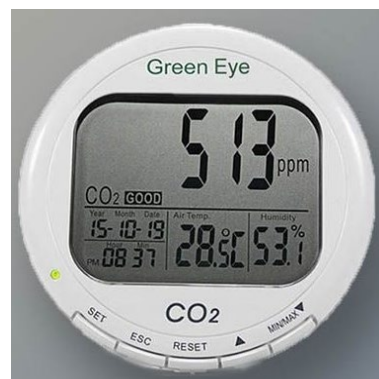
Figure 3.6. The data logger, Green Eye – Desktop Environmental Monitor
